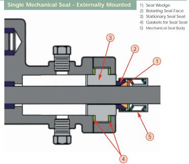
The **External Mechanical Seal** arrangement is used when system pressures are below atmospheric pressure (vacuum). This is because the atmospheric pressure will assist in holding the seal faces together. This seal arrangement isolates the mechanical seal from the fluid being pumped which can be an advantage when pumping chemicals that are not compatible with the seal body. The maximum fluid viscosity recommended is 5000 CPS.
