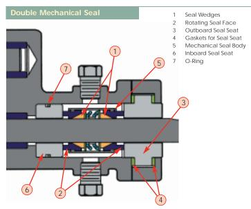
The **Double Mechanical Seal** arrangement relies on a lubricating system to cool the seal faces. The lubricating barrier liquid washes the seal faces and must be safe and compatible with the pumpage. Accordingly, double seals are preferred for crystallizing or abrasive liquids as the seal faces are only exposed to the flush liquid. Double seals must be pressurized so that the seal chamber has about 15 PSI higher pressure than the pump discharge pressure.
